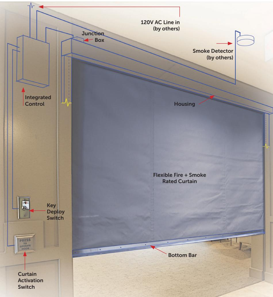
**System Operation.** The system is deployed on an alarm signal from the local smoke detector or from a fire control panel. System power requirement is 120 VAC. The unit is also equipped with a 24 VDC battery back-up system that is maintained by the electronic controls. When required, the system can also be connected to building standby power. The controls include a universal power supply that can be adapted to foreign electrical current requirements.
